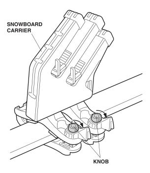
9. Return the cam levers to the original location (turn clockwise).
