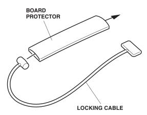
14. Insert the locking cable plate into the slit of the snowboard carrier. To carry one snowboard, insert the plate into the lowest slot. To carry two snowboards, use one of the upper three slots in the carrier.
