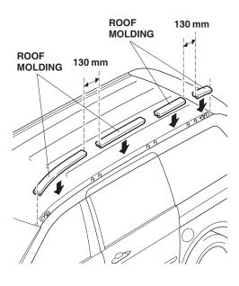
7. Place the left center stay over the two stud bolts at the center of the roof, and install the two TORX nuts using a T-30 TORX driver. Torque the TORX bolts to 5 to 8 lb-ft. (7 to 10 N·m).
