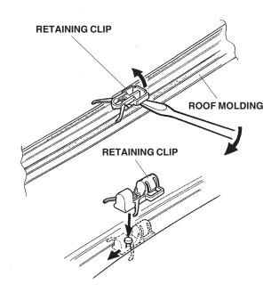
4. If any of the six center retaining clips remained on the roof, remove them from the stud bolts using long nose pliers.
