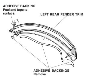
9. Using an alcohol swab, throughly clean the area where the left rear fender trim will attach. Align the edge of the left rear fender trim with the bumper seam as shown. While applying light pressure against the rear fender trim, carefully remove the taped adhesive backing.
