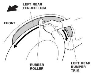
13. Hold the left rear fender trim upward and bend the mounting tabs around the left rear fender. Use needle-nose pliers wrapped in a shop towel to bend the mounting tab around the fender flange. Repeat for the left rear bumper trim.
