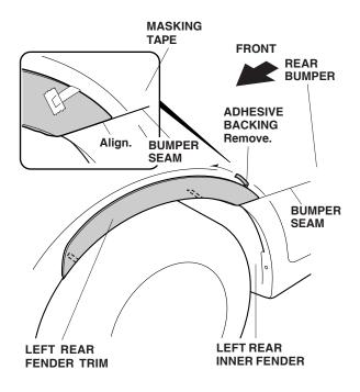
10. Peel back the adhesive backing from the upper part of the left rear bumper trim and tape it to the surface. Remove the remaining adhesive backings from the left rear bumper trim.
