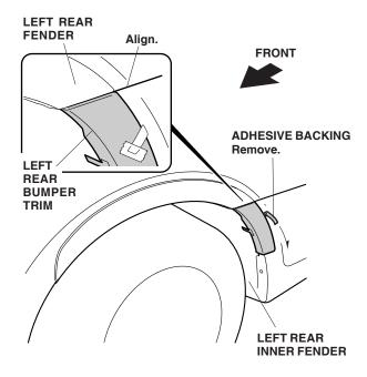
12. Using a rubber roller, apply pressure against the fender trim and roll from one end to the other.
