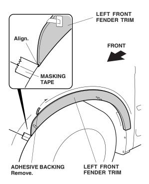
4. Attach the left front fender trim to the left front fender. While applying light pressure against the left front fender trim, carefully remove the taped adhesive backing.
