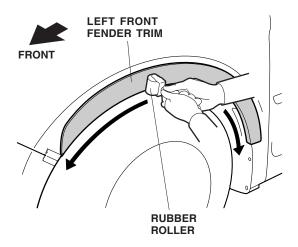
Hold the left front fender trim upward, and push
