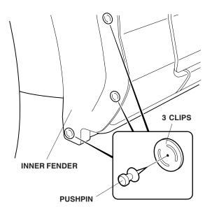
Using a pushpin, make a hole through the centers of the three fenderwell clips.
