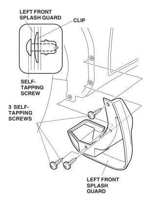
4. Turn the steering wheel all the way clockwise and install the right front splash guard the same way.
