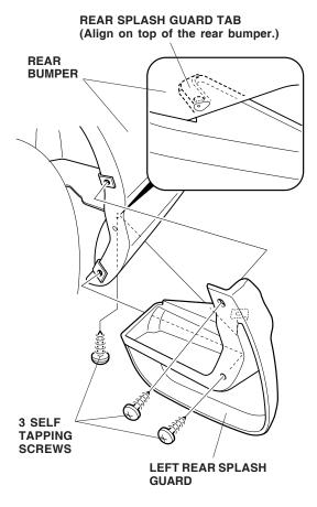
9. Tighten the self-tapping screws securely in the order of 1, 2, and 3.
