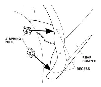
6. Slide one spring nut over the hole in the left rear splash guard. Pay attention to the installation direction of the spring nut.
