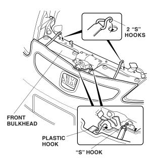
11. Attach the four "S" hooks to the grille opening. Insert the two tabs between the grille and the front bumper, and attach the four plastic hooks to the bottom edges of the front grille.
