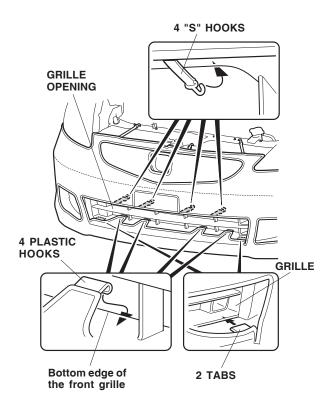
12. Route the elastic cord through the loops on the bottom of the mask and attach the hooks at the ends of the elastic cord to the bottom of the bumper on both sides.
