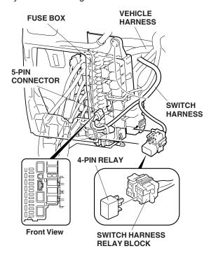
39. Plug the switch harness 5-pin connector into the 5-pin slot of the fuse box.
