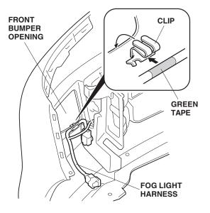
24. Route the fog light harness along the front bumper to the right side of the vehicle and attach the five fog light harness clips to the five ribs inside the front bumper. If necessary, remove the upper air screen screw.
