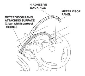
14. After installing the panel, use the palm of your hand to hold pressure against it for 30 seconds.
