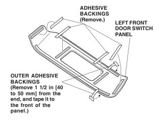
2. Remove and discard the inner adhesive backings and the small pieces of outer adhesive backings. Attach a strip of masking tape to the end of each remaining outer adhesive backing, and remove 1 1/2 in (40 to 50 mm) of the adhesive backing. Fold the ends back, and tape them to the front of the panel.
