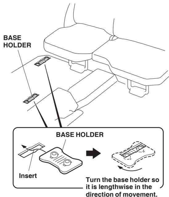
16. Place one hook holder over each base holder with the arrow on the hook holder facing forward. Push down to snap the hook holders and base holders together, making sure they are completely joined.
