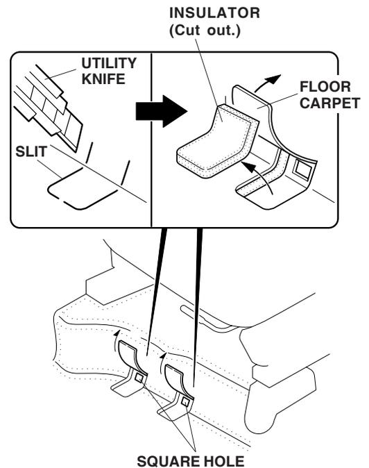
2. Make cuts with a utility knife at the slits in the floor carpet at the two locations shown.
