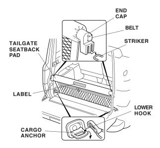
2. Attach the tailgate seat back pad lower hooks to the left and right lower anchors on the vehicle.
