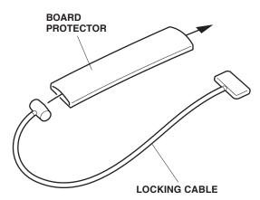
14. Insert the locking cable plate into the slit of the snowboard carrier. For one snowboard, insert the plate into the lowest slit. For two snowboards, use one of the upper three slits in the carrier.
