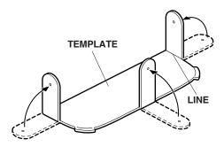
2. Fit the template on the right side of the roof glass along the seal line, insert two tabs into the gap between the roof glass and the seal, and secure the template with masking tape.
