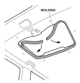
10. Gently pull down the roof lining and install one snap screw, two washers and one flange nut in each of the six holes you made.
