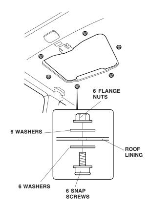
11. Reinstall the molding placing it over the roof panel and roof lining.
