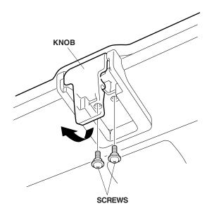
8. Release the tab and remove the skylight opener cover.
