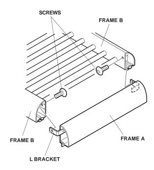
Install the remaining frame A to frame B the same way. 7. Slide four of the eight square nuts into frame B through the groove shown. Repeat on the other frame B.
