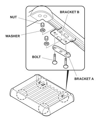
11. Position the roof basket on the roof rack, with the flap from frame A facing forward. Attach the basket to the cross bars by sliding bracket A around the crossbar and tightening the nuts evenly.
