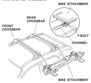
Turn and adjust the mounting lever to lock the bike attachment to the roof rack. Check for firm pressure while you push down on the mounting lever to lock it into place.
