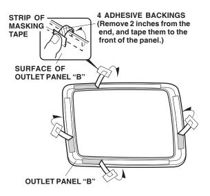
10. Position the outlet panels "A" and "B" on the existing outlet panels. While holding pressure on the outlet panels, carefully remove the adhesive backings from the outlet panels. Press the outlet panels "A" and "B" firmly against the existing outlet panels with the palm of your hand, particularly at the edges for 30 seconds.
