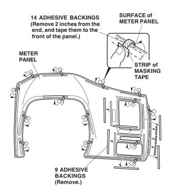
3. Position the meter panel on the existing meter panel. While holding pressure on the meter panel, carefully remove the adhesive backings from the meter panel. Press the meter panel firmly against the existing meter panel with the palm of your hand, particularly at the edges for 30 seconds.
