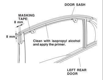
11. When the isopropyl alcohol is dry, carefully apply primer to the door sash. Wipe off any excess primer immediately. Allow the primer to dry for at least 3 minutes.
