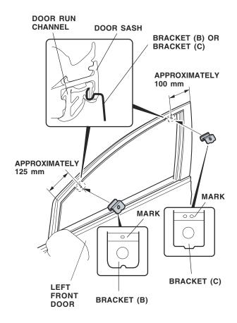
19. Install a bracket (B) and a bracket (C) on the door sash at the measurements shown. Verify the shape and the identification mark stamped on each bracket. Be sure to use the correct bracket at the proper location. 20. Hook the front bracket from the left front door visor on the door sash, and install it so that there is no space between the bracket and the door sash.
