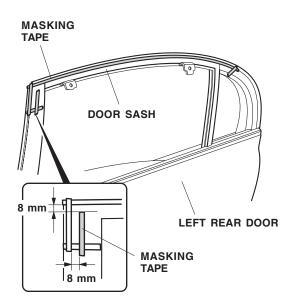
10. Using isopropyl alcohol on a clean shop towel, clean the area where the visor will attach.
