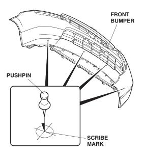
4. While wearing eye protection, drill a 10 mm hole through each marked location from the outside of the bumper. First drill with a 3 mm bit, and finish with a 10 mm bit. Remove any burrs from the edges of the holes with a file.
