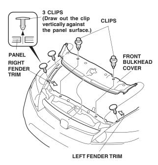
With the help of an assistant, remove the front bumper (four bolts, four long clips fastening the front bumper and air spoiler, six clips, and two self-tapping screws). Unplug the fog light and/or the front corner sensor connectors, if equipped. Place the front bumper on a blanket to install the front under spoiler. Do not remove the clips fastening the air spoiler.
