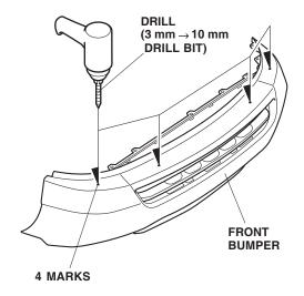
5. While wearing eye protection, drill a 3 mm hole through the four dimpled areas of the front bumper on both sides. Remove any burrs from the edges of the holes with a file.
