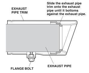
Using the torque wrench, tighten the flange bolt to the specified torque.
