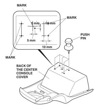
5. While wearing eye protection, drill four 5 mm holes and one 30 mm hole through the marks you just made.
