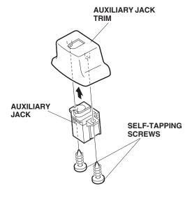
8. Position the auxiliary jack on the pocket of the center console cover, and install the four self-tapping screws.
