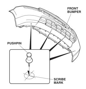
4. While wearing eye protection, drill a 10 mm hole through each marked location from the outside of the bumper. First drill with a 3 mm bit, then finish with a 10 mm bit. Remove any burrs from the edges of the holes with a file.
