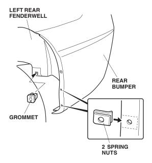
7. Position the left rear splash guard on the left rear fenderwell and rear bumper, then install the three 5 x 20 mm self-tapping screws. Tighten the three self-tapping screws in the order shown. Cut off any excessive undercoat material with a utility knife.
