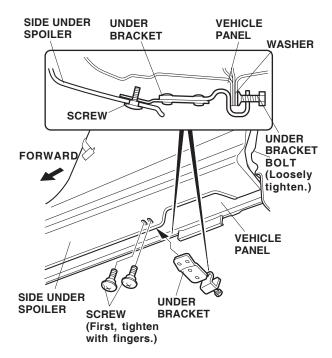
Position the under bracket on the side under spoiler and loosely install the two screws. Tighten the under bracket bolt, but don't tighten it completely yet. 31. Align the rear top edge of the left side under spoiler with the edge of the radius of the vehicle panel as shown. Remove the five adhesive tapes from the left side under spoiler. Press firmly on the side under spoiler firmly.
