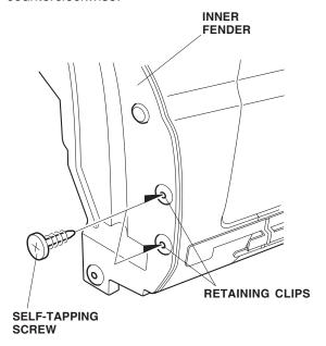
20. Using a self-tapping screw, pierce a hole through the center of the inner fender retaining clips.
