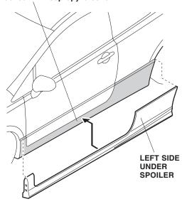
2. Using a tape measure and felt-tip pen, measure and mark the body as shown.
