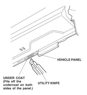
26. Apply touch-up paint to the vehicle panel in the area where you filed off the undercoat. Do not install the under bracket until the touch-up paint drys. 27. Gently tap on the left side under spoiler to remove any gap between the spoiler and the wheel arch.
