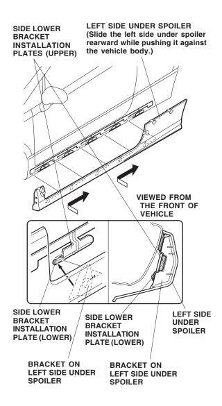
23. Check that all six brackets on the left side under spoiler are set in the side lower bracket installation plates. Visually check that there is no excessive gap between the left under spoiler and the vehicle. If an excessive gap is found, repeat step 22.
