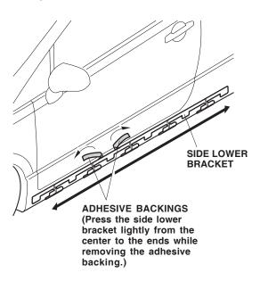
When the workshop room temperature is below 60°F (15°C), warm up the entire side lower bracket to 60°F (15°C) or above before attaching it to the vehicle body.
