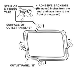
10. Position the outlet panels "A" and "B" on the existing outlet panels. While applying pressure to the outlet panels, carefully remove the adhesive backings from the outlet panels. Press the outlet panels "A" and "B" firmly against the existing outlet panels with the palm of your hand, particularly at the edges.
