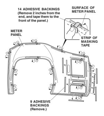
Position the meter panel on the existing meter panel. While applying pressure to the meter panel, carefully remove the adhesive backings from the meter panel. Press the meter panel firmly against the existing meter panel with the palm of your hand, particularly at the edges.
