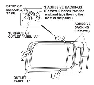
8. Attach a strip of masking tape to the end of each shaded adhesive backing. Peel back 2 inches (5–6 cm) of the adhesive backings, and fold them over as shown. Temporarily attach strips of masking tape to the outside of the outlet panel "A". Remove all remaining adhesive backings from the outlet panel "A".
