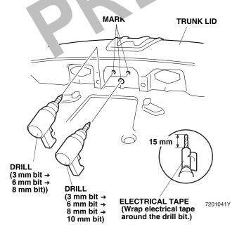
27. Install two well-nuts into the 8 mm holes.
