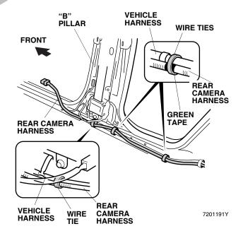
47. Route the rear camera harness through the passenger's door opening, and secure it to the vehicle harness with five wire ties.
