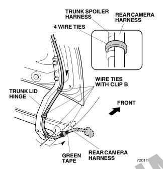
41. Route the rear camera harness towards the rear of the vehicle, and secure it to the vehicle panel hole with one wire tie with clip A.
