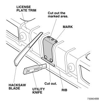
57. Using a utility knife, cut out the rib from the license plate trim as shown.
