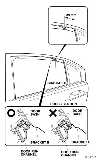
11. Install bracket B to the door sash at the measurement shown. Verify the shape and the identification mark stamped on the bracket. Be sure the door run channel is installed properly before installing the bracket.
