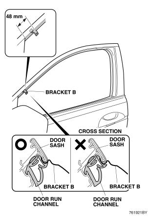
2. Install bracket B to the door sash at the measurement shown. Verify the shape at the identification mark stamped on the bracket. Be sure the door run channel is installed properly before installing the bracket.
