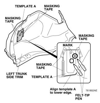
7. Using a felt-tip pen, mark the left trunk side trim as indicated on the template. Remove the template.
