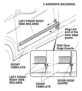
7. Peel back approximately 1-1/2 to 2 inches of the adhesive backing from each adhesive tape, and tape the ends to the outside surface of the molding. Remove the other adhesive backings.
