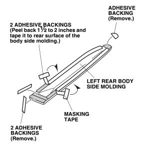
8. Align the end of the left rear body side molding with the rear template as shown and temporarily attach it along the top edge of the rear template.
