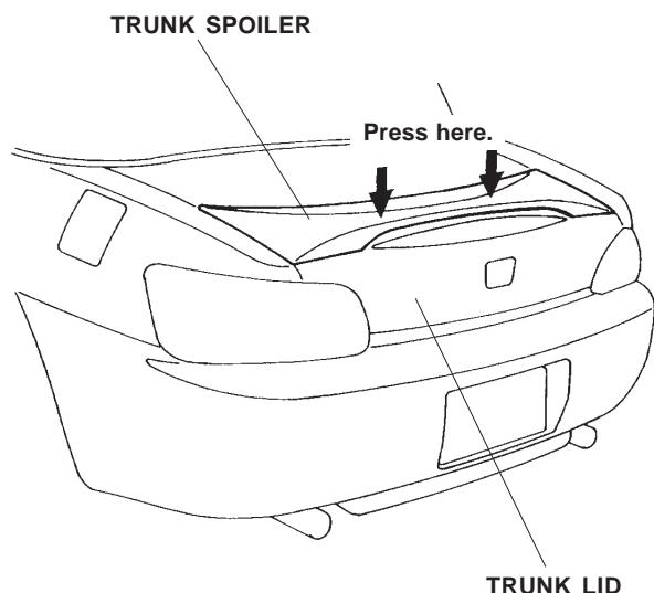
8. Slowly remove the trunk spoiler from the trunk lid. Check that the marking washers stay attached to the trunk lid.
