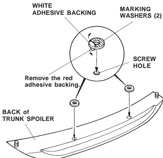
6. Remove the white adhesive backings from the marking washers. With the trunk lid closed, insert the studs from the trunk spoiler into the holes in the trunk lid.
