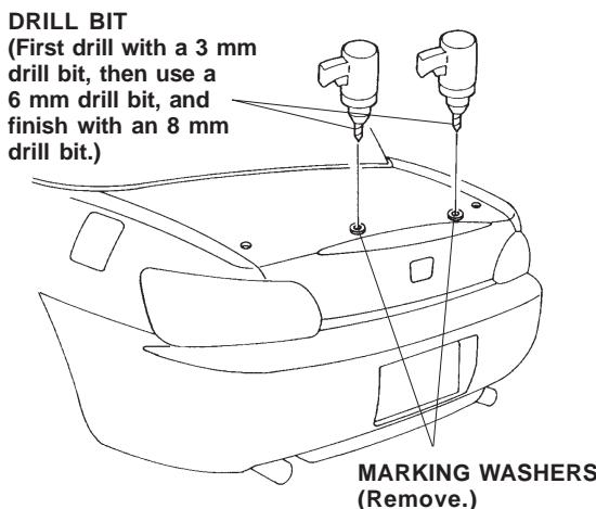
10. While wearing eye protection, drill an 8 mm hole through each center-punched mark:
