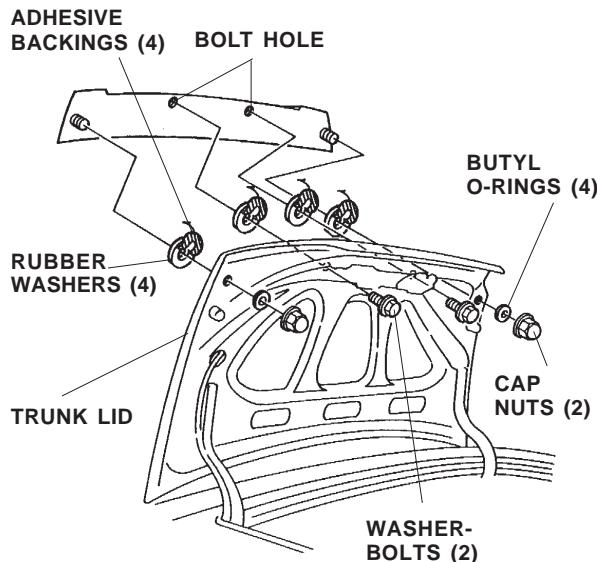
12. Fit the trunk spoiler into position on the trunk lid. Install a butyl O-ring and a cap nut on the end of each stud, but don't tighten the cap nuts yet.
