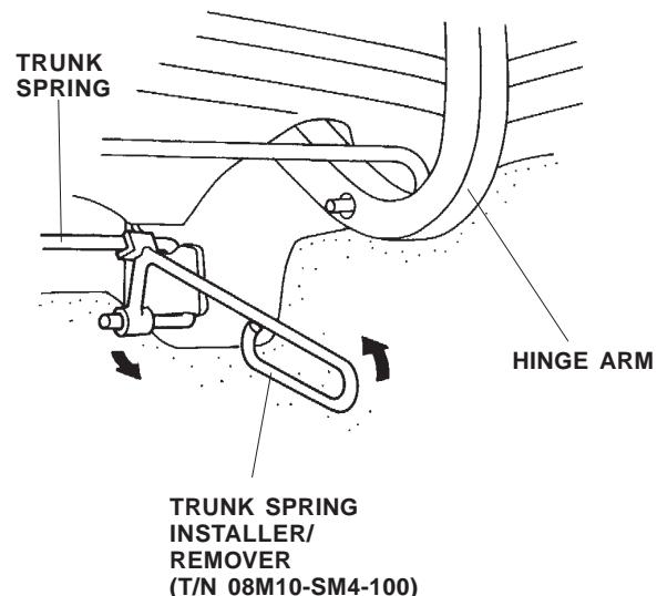
16. Install the heavy-duty springs in the reverse order of removal:
