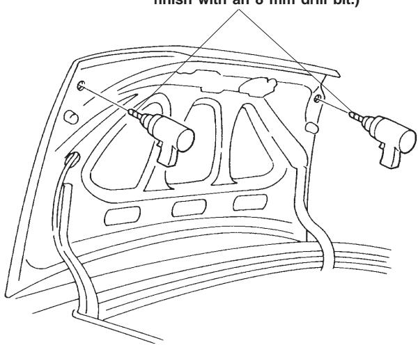
5. Remove the red adhesive backings from the two marking washers, and attach them to the trunk spoiler over the two screw holes.
