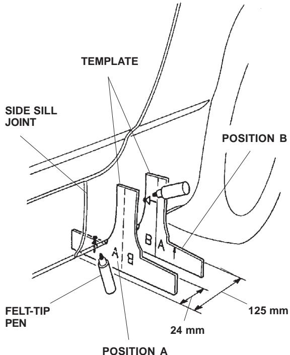
4. Use the tape measure to measure 125 mm toward the rear of the side sill joint. Turn the template around, and position the template on the side sill as shown in position B. Using a felt-tip pen, mark the side sill in position B. To ensure that the holes will be in the correct position, keep the template straight.
