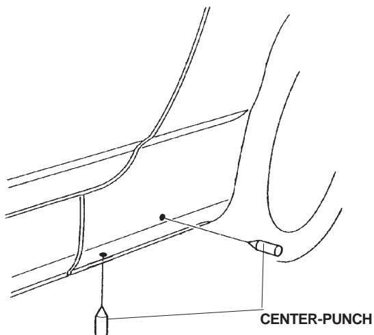
6. While wearing eye protection, drill an 8 mm hole through the upper center-punched mark:
