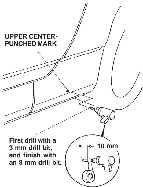
7. While wearing eye protection, drill a 10 mm hole through the lower center-punched mark:
