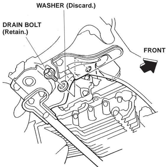
4. Install the new aluminium washer and the engine block heater into the bolt hole using a 24 mm socket and a torque wrench. Torque the engine block heater to 60 N·m (44 lb-ft).
