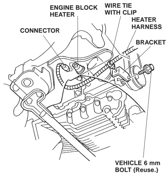
7. Remove the 6 mm bolt that fastens the engine front cover, and attach the bracket from the kit with this 6 mm bolt. Torque the 6 mm bolt to 12 N·m (9 lb-ft).
