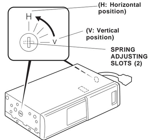
13. Position the side bracket included in the CD changer kit on the CD changer, and install four of the 4 x 6 mm washer-screws also provided with the CD changer kit.
