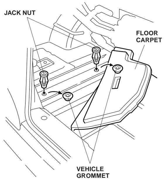
11. Thread a flange-bolt into each of the jack nuts with the special tool provided:
