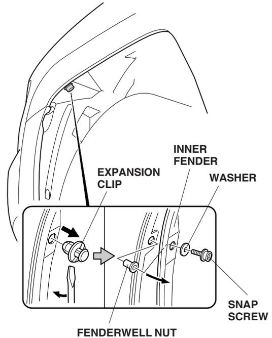
4. Pull the inner fender back, and press one fenderwell nut (supplied) into the hole in the fender flange.
