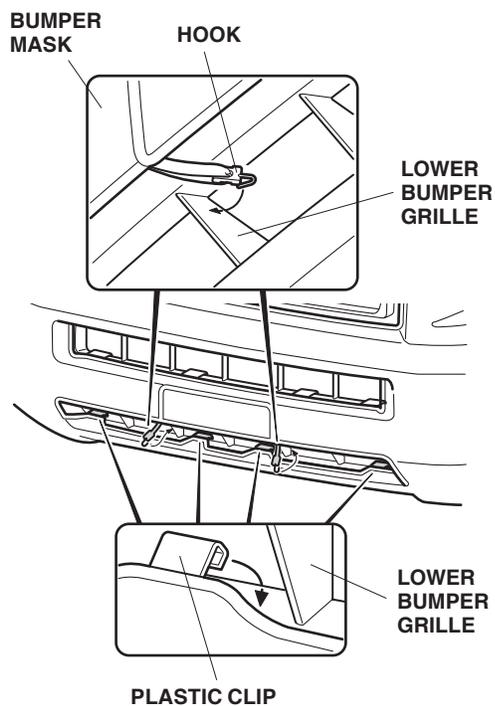
16. Attach the six hooks to the bottom inside edge of the front bumper.
