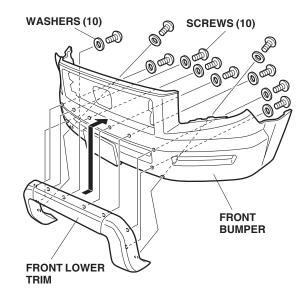
4. Reinstall the front bumper. Check that all retaining tabs and clips are installed properly without play or rattle.
