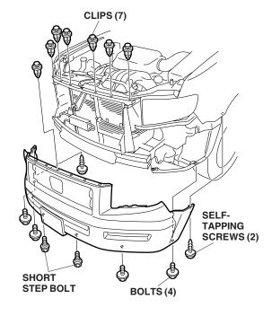
2. Remove the existing front grille (nine self-tapping screws and eight tabs).
