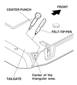
11. While wearing eye protection, drill an 8 mm hole through the center-punched mark on the left side of the tailgate. Use a drill stop to avoid drilling through the inner panel. First drill with a 3 mm drill bit, and finish with an 8 mm drill bit. After drilling, remove all burrs from the edges of the hole with a file.
