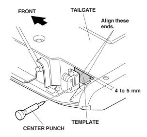
10. Using the felt-tip pen and the center punch, mark the right side of the tailgate at the center of the triangle area.
