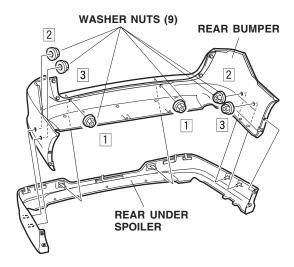
11. Install the five long stepped bolts through the inboard holes in the under spoiler, and install the four short stepped bolts through the outboard holes in the under spoiler. Install a washer-nut on each stepped bolt. Tighten the washer-nuts in the order shown.
