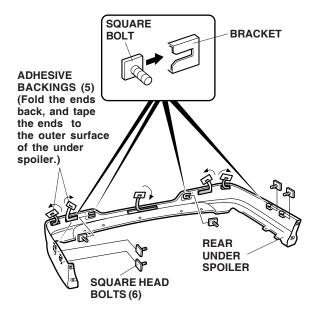
6. Attach a strip of masking tape to the end of each adhesive backing, then pull back 1½ to 2 inches of adhesive backing. Fold the ends back, and tape them to the outer surface of the spoiler with masking tape.
