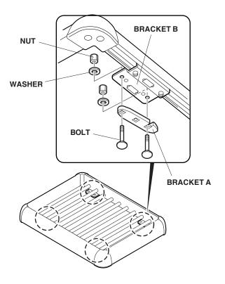
11. Position the luggage basket on the roof rack, with the flap on frame A facing forward. Attach the basket to the cross bars by sliding bracket A around the crossbar and tightening the nuts. Tighten the nuts evenly.
