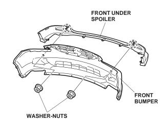
13. Secure the front bumper to the front under spoiler using the five stepped bolts.
