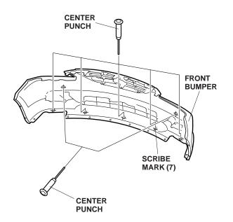
5. While wearing eye protection, drill two 8 mm holes through the front bumper. First drill with a 3 mm drill bit, then finish with an 8 mm drill bit.
