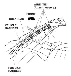
50. Route the fog light harness behind the battery, and loosely secure it to the vehicle harness with three additional wire ties.
