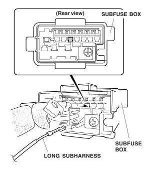
25. Secure the long subharness to the subfuse box harness with one small wire tie.
