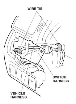
74. Locate the 2-pin connector at the front of the fuse box that is black-taped to the vehicle harness near the front bulkhead. Remove the black tape to free the connector. Plug the 2-pin connector from the switch harness into the vehicle harness 2-pin connector you just freed.
