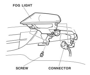
3. Remove the screw that fastens the fog light, and pull the light out toward you.
