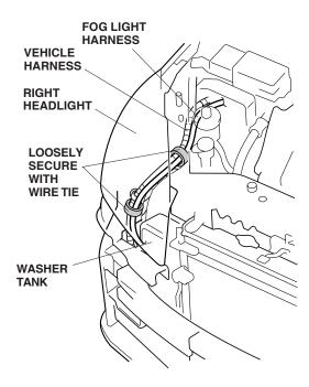
41. Route the right fog light harness 2-pin connector along the vehicle harness and into the bumper area.
