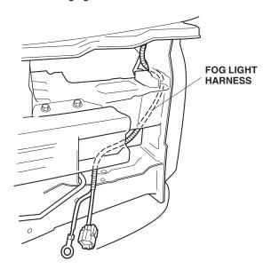
54. **EX model with AUTO air:** Secure the fog light harness to the sensor harness with three wire ties.
