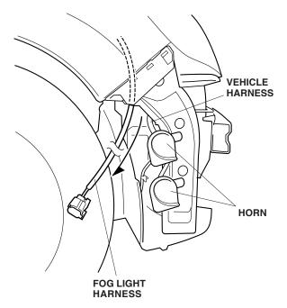
42. Attach the two wire ties with clips on the fog light harness into the holes in the vehicle body.
