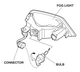
Install the new bulb into the fog light. Align the tab
