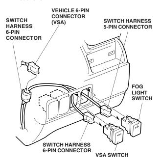
72. Route the 6-pin switch harness connector through the switch hole and plug it into the VSA switch. Plug the vehicle 6-pin VSA connector into the switch harness.
