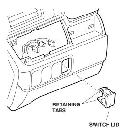
68. Remove the VSA switch. (two retaining tabs).
