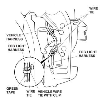
45. Tighten the two wire ties installed in step 40.
