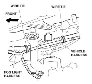
49. Route the fog light harness along the vehicle harness on the bulkhead, and loosely attach the fog light harness to the vehicle harness with four wire ties.
