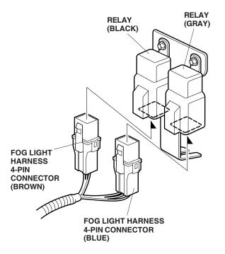
62. Loosen the bolt that secures the existing relay box, and slide the tab from the fog light relay bracket under the bolt. Retighten the relay bracket bolt.
