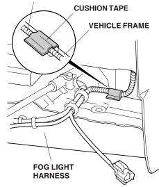
59. Tighten the seven wire ties installed in steps 49 and 50.
