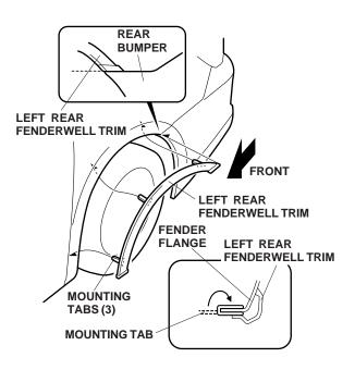
9. Using a rubber mallet, install the inner protector over the fender flange and fenderwell trim.
