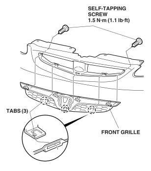
Position the front grille on the front bumper by installing the three lower retaining tabs into the front bumper and reinstall the two self-tapping screws removed in step 2. 6. Align the upper edge of the front grille with the upper edge of the front bumper by pushing down on the front grille, then while remove the adhesive backings, and use the palm of your hand to hold pressure against it for 30 seconds. Start from the center and work toward the sides.
