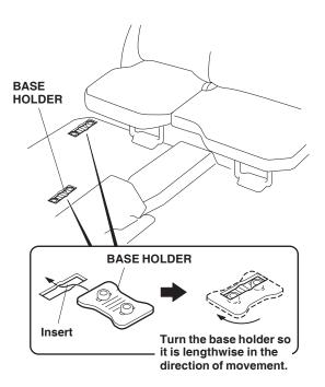
16. Place one hook holder over each base holder with the arrow on the hook holder facing forward. Push down to snap the hook holders and base holders together, making sure they are completely joined.
