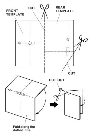
11. Fold each template along the dotted lines. Using scissors, cut the dashed lines to remove the circle from each of the templates.
