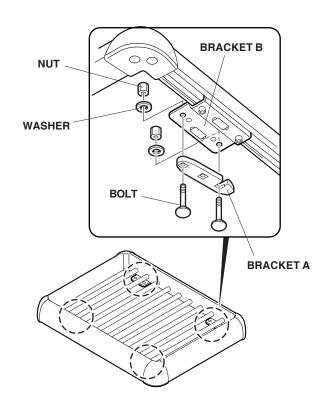
11. Position the roof basket on the roof rack, with the flap from frame A facing forward. Attach the basket to the cross bars by sliding bracket A around the crossbar and tightening the nuts evenly.
