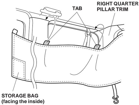
17. Slide the remaining tab into the rear door striker cover. If you are also installing the front privacy curtain, cross the tabs so that both curtains overlap each other, and secure it with the velcro straps as shown.
