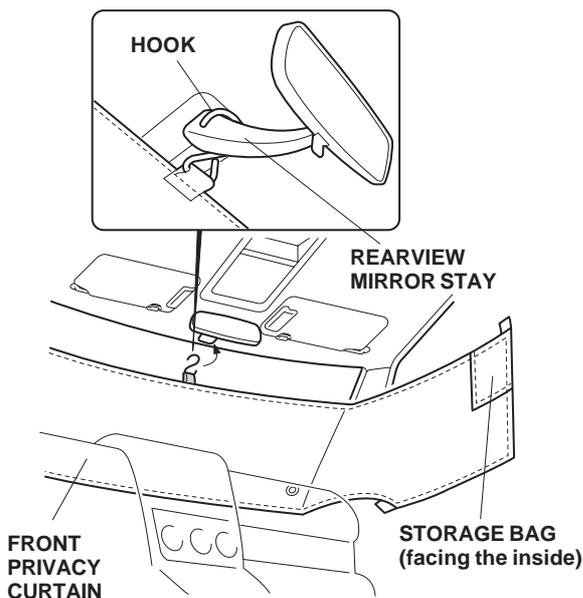
3. Spread the privacy curtain over the right front windshield and passenger's window. Slide the two tabs into the instrument panel and rear door striker cover.
