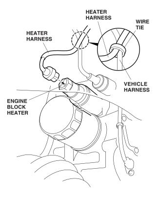
Route the heater harness alongside the vehicle harness and secure the heater harness to the vehicle harness, with three wire ties in the areas shown.
