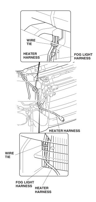
14. Route the heater harness out through the front bumper grille. Continue routing the heater harness through the back of the bumper ribs, then secure it to the ribs with two wire ties as shown.
