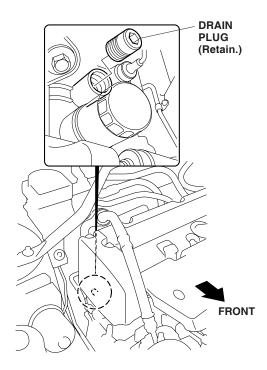
6. Install the engine block heater with the aluminum washer into the bolt hole using a 24 mm socket and a torque wrench. Torque the engine block heater to 60 N·m (44 lbf-ft).
