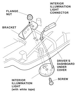
32. Bundle the ambient light harness and secure the connector to the bracket using a wire tie with clip.
