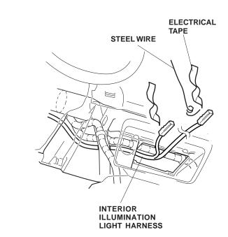
20. Remove the wire and electrical tape from the interior illumination light harness.
