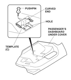
40. Using a pushpin, pierce the template at the three marked points. Remove the template.
