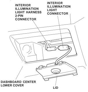
57. Plug the interior illumination light harness 2-pin connector to the interior illumination light connector on the passenger's dashboard under cover, and reinstall the under cover.
