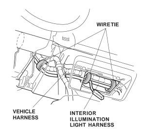
24. Secure the interior illumination light harness to the vehicle harness using four wire ties if the vehicle is equipped with the driver's dashboard under cover. Use three wire ties if the vehicle is without the driver's dashboard under cover.
