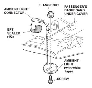
43. Wrap another piece of the EPT sealer that you cut into three equal pieces around the interior illumination light connector.
