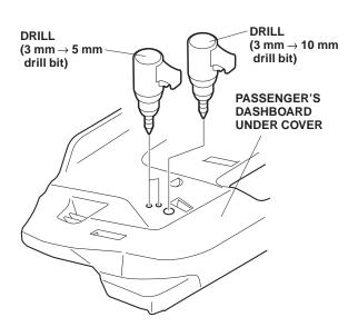
42. Route the interior illumination light (with white tape) connector through the 10 mm hole. Install the interior illumination light on the passenger's dashboard under cover with the screw and flange nut.
