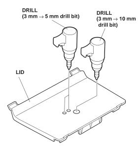
37. Route the interior illumination light (with blue tape) connector through the 10 mm hole. Install the courtesy light on the lid with the screw and flange nut.
