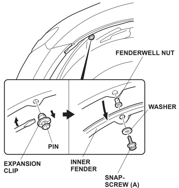
6. Pry out the plastic pin, and remove the expansion clip that fastens the inner fender. Remove and retain the clip, then clean the area around the hole.
