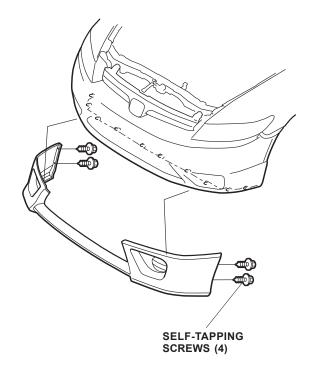
6. While holding pressure on the front under spoiler, carefully remove the adhesive backings in the sequence shown. After removing, hold the front under spoiler firmly against the front bumper with the palm of your hand for 30 seconds. Tighten the self-tapping screws installed in step 5.
