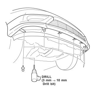
8. Secure the front under spoiler to the front bumper with seven flange-nuts and seven flange bolts.
