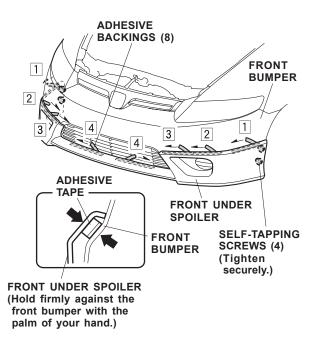
7. Locate the seven front under spoiler brackets. Mark the front bumper with a pushpin through the center of the hole in each bracket. Using a drill, drill a 10 mm hole through each marked location. First drill with a 3 mm bit, and finish with a 10 mm bit. Remove any burrs from the edges of the holes with a file.
