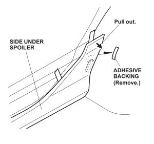
29. Remove the three adhesive tapes from the left side under spoiler. Press on the adhesive part of the side under spoiler firmly.
