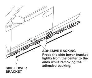
When the workshop room temperature is below 60°F(15°C), warm up the entire side lower bracket to 60°F(15°C) or above before attaching it to the vehicle body.
