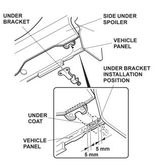
22. Cut into the marked area of the under coat with a utility knife, and file off the under coat from the surface side and inner side of the vehicle panel.
