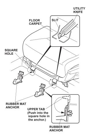
Push the lower tab of the anchor into the square hole concealed under the floor carpet. Pull the upper tab down, and push it into the square hole in the anchor as shown. Repeat on the remaining anchor. 4. Install the driver's side rubber mat by placing the rings in the rubber mat over the anchor pins.
