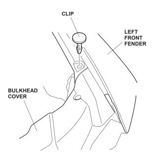
3. Install one new clip with a snap-screw(B) into the hole where you removed the clip, and tighten the snap-screw(B).
